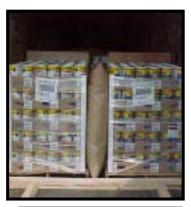
Lading unitized with stretch wrap to the pallet and braced by floor blocking and DID bag
